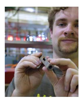
SLAC physicist Andrew Fisher holds a section of heavy copper winding used as a conductor in electromagnets, hollowed out to carry low conductivity cooling water.
