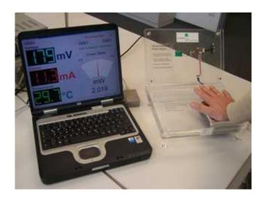
New circuits transform body heat – such as that of a hand – into electricity. © Fraunhofer IIS
