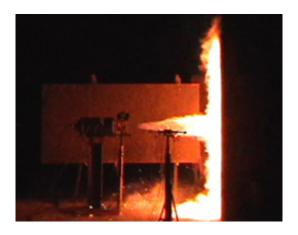
The experiment shown in this image helps Sandia scientists understand the hazards associated with an unintended release of hydrogen. It shows the flame that emerges after a high-pressure jet of hydrogen is released toward a wall made of cinder block. The radiated heat flux emanating from the flames, when analyzed and measured, helps researchers evaluate the effectiveness of a barrier wall in mitigating the risks of hydrogen releases in a dispensing station setting. Credit: SNL
