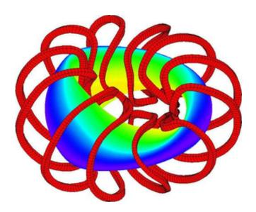
Stellarator design with 12 twisted coils that generate an external magnetic field to confine the plasma. The color map of the plasma displays an axial symmetry property of the magnetic field strength that enhances confinement. Credit: Alexander, et al. ©2007 PNAS.
