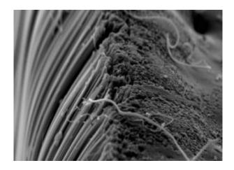
These spaghetti-like structures are carbon nanotubes viewed under an electron microscope. The manufacture of these nanotubes can produce toxic byproducts, researchers report. Credit: Photo by Anastasios John Hart
