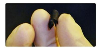
A sample of the new nanocomposite paper developed by researchers at Rensselaer Polytechnic Institute. Infused with carbon nanotubes, the paper can be used to create ultra-thin, flexible batteries and energy storage devices for nextgeneration electronics and implantable medical equipment. Credit: Rensselaer/Victor Pushparaj
