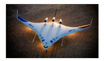
Boeing's X-48B Blended Wing Body technology demonstrator shows off its unique lines at sunset on Rogers Dry Lake adjacent to NASA Dryden Flight Research Center. Credit: NASA
