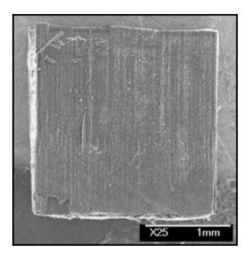
The same carbon nanotube block after being compressed more than 500,000 times. Even after this stress, there is virtually no difference in the block's shape, mechanical integrity or electrical conductivity. This resistance to wear and tear is similar to the behavior of soft tissues such as a shoulder muscle or a stomach wall.Credit: Rensselaer/Victor Pushparaj
