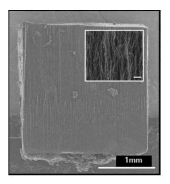
A two-millimeter square block of carbon nanotubes, made up of millions of individual, vertically aligned, multiwalled nanotubes. Credit: Rensselaer/Victor Pushparaj
