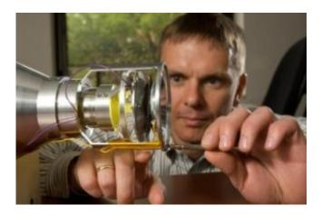
NSCL assistant professor Krzysztof Starosta adjusts a device designed by Alfred Dewald, an NSCL user from the University of Cologne, that is capable of making highly precise in-flight distance measurements on the sub-micron scale. (A micron is one-millionth of a meter.) The device was used in a first-of-its kind experiment for fast-beam rare isotope research laboratories such as NSCL. Credit: National Superconducting Cyclotron Laboratory
