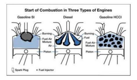
In a gasoline spark-ignition engine (left), combustion begins when a mixture of fuel and air is ignited by the spark plug. In a diesel engine (center), combustion begins when fuel is injected into hot, highly compressed air. In a homogeneous charge compression ignition engine (right), well-mixed fuel and air are compressed until combustion occurs at multiple points throughout the combustion chamber. Diagram courtesy / MIT Laboratory for Energy and the Environment
