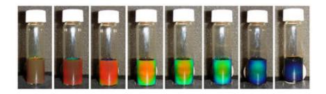
Image shows the solution of iron oxide in water changing color under a magnetic field, with increasing strength of the field from left to right. Photo credit: Yin laboratory, UCR
