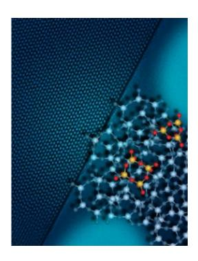
On the left is a TEM micrograph of a porous, cube-like nanostructure. On the right is a blow-up of the silica framework (the dark
