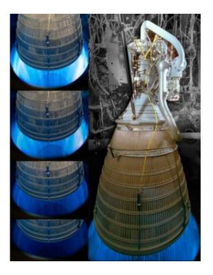
The Common Extensible Cryogenic Engine, or CECE, is a liquid oxygenhydrogen pump-fed engine developed to demonstrate advanced rocket technologies for future space vehicles. (Pratt & Whitney Rocketdyne)
