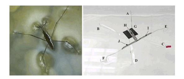
(Left) Photo of the water strider insect. (Right) Photo of the 1-gram robot on the surface of the water. A, B, C, D: supporting legs; E and F: actuating legs; G: body with on-board electronics and power source; H: middle actuator; I and J: right and left actuators. Image credit: Yun Seong Song and Metin Sitti. ©IEEE 2007.
