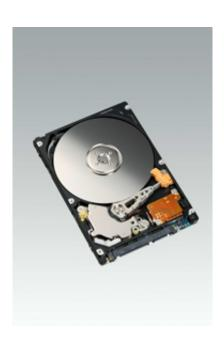
Fujitsu Limited today announced that it has developed the new MHY2 BS Series of 2.5" hard disk drives, which are designed for 24-hour continuous operation and are available in storage capacities of up to 200 GB. Sales of the new series will start at the end of August.
