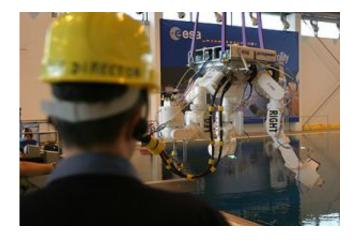
Eurobot is lowered into the Neutral Buoyancy Facility at the European Astronaut Centre (EAC), in Cologne, Germany. Under the watchful eye of the Test Director, Hervé Stevenin, the Eurobot WET model is lowered into the pool ahead of testing to verify the operational concept for Eurobot. Credits: ESA
