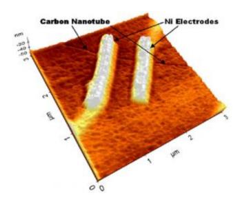
UT Dallas researchers are using nickel electrodes to explore making electrical contact with a carbon nanotube that is about one-100,000th the width of a human hair. Credit: University of Texas at Dallas
