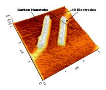
UT Dallas researchers are using nickel electrodes to explore making electrical contact with a carbon nanotube that is about one-100,000th the width of a human hair. Credit: University of Texas at Dallas
