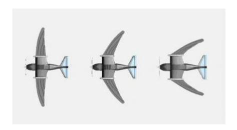
RoboSwift can sweep its wings back and forth, changing the shape and the surface area. By doing so the airplane can fly more efficiently and more agilely than fixed-wing aircraft. The airplane is powered by means of a special propeller that folds during gliding to minimize air drag. Credit: RoboSwift team
