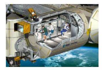
An artist's impression of Columbus, a cutaway view, the European laboratory module of the International Space Station. Credits: ESA - D.Ducros
