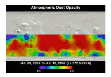
The map shows the atmosphere's opacity at an infrared wavelength of 9 micrometers. The scale bar's values run from nearly clear (0.05) to roughly a two-thirds reduction in sunlight (0.40).Image credit: NASA/JPL/Arizona State University
