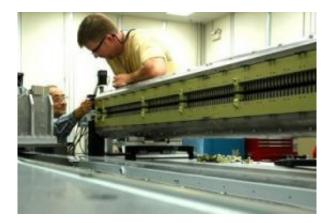
Preparation -- Isaac Vasserman (left) and Matt Kasa of Argonne's Accelerator Systems Division prepare an undulator for magnetic tuning and verification. Credit: Argonne National Laboratory
