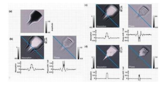
A tungsten tip is iteratively reconstructed as a hologram: (a) normalized hologram (b) conventional reconstruction yields reconstructed absorption and phase distributions (c) first iteration makes oscillations due to twin image apparent in these reconstructions (d) after the 500th iteration. Credit: Hans-Werner Fink, Reprinted with permission from Phys. Rev. Lett. Vol. 98, 233901 (2007). Copyright 2007 by the American Physical Society. (http://link.aps.org/abstract/PRL/v98/e233901)
