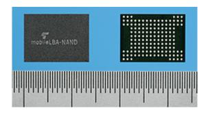
Toshiba Corporation today announced a new series of embedded NAND Flash memories for mobile phones offering both a configurable single-level cell (SLC) memory area and a multi-level cell (MLC) memory area, allowing applications and data to be stored on the same chip.
