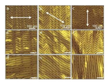
Images of the stretchable silicon membrane (a,b,c) The membrane in the relaxed state before stretching in the horizontal, diagonal, and vertical directions, respectively (d,e,f) The membrane during stretching in these directions (g,h,i) The membrane at full stretch. Credit: John Rogers
