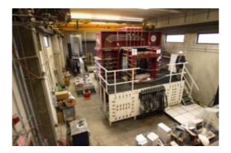
Standing more than 15 feet tall at two stories, weighing nearly 40 tons and containing more than a mile of pipes to transport oil pressure to its 40 jacks, the "Universal Element Tester" measures the strength of reinforced concrete under earthquake-like conditions. Civil Engineering Professor Thomas Hsu (pictured) and his colleagues designed and built this one-of-a-kind machine housed at UH. Credit: Todd Spoth
