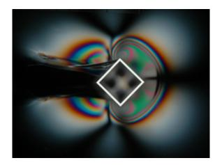
Birefringent visualization of the micellar fluid layer around a diagonally oriented square "cutting tool." A white outline is superimposed on the outer edge of the square.
