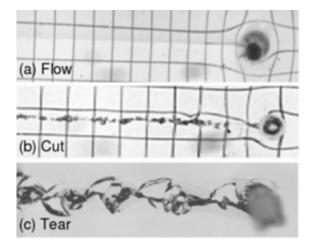
Responses of a micellar fluid to a cylinder moving at three speeds: (a) 2.8 mm/s, d=3.1 mm; (b) 9.9 mm/s, d=1.8mm; (c) 16 mm/s, d=7.9 mm. The view shown is along the cylinder axis.
