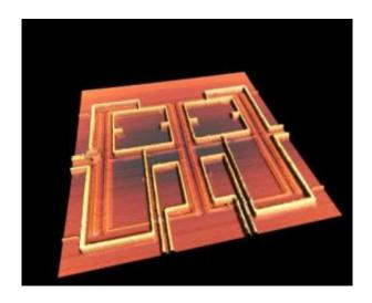
Superconducting rings on a chip. Credit: TU Delft
