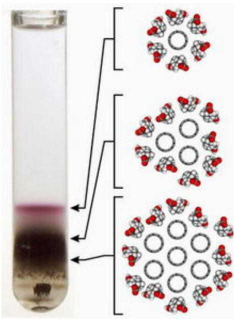
The vial holds a nanotube solution after ultracentrifuging has separated it into different layers. The purple layer at the top consists of a highly uniform population of the single-walled semiconductor nanotubes that are the most strongly luminescent. The illustrations at the right show the typical constituents of each layer. Credit: Tobias Hertel
