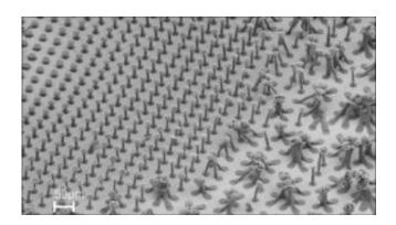
Nanotube height, diameter and spacing affect the densification process. If the nanotube bundles are too short, like those on the left, there is no densification at all. If the bundles are too tall, like those on the right, bundles are not rigid enough and tend to stick with one another after densification. The middle region, where bundles are between 30-65 micrometers tall, demonstrates good densification. Credit: Rensselaer/Liu
