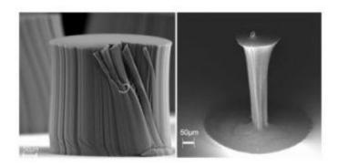
A carbon nanotube bundle before (left) and after (right) densification. Credit: Rensselaer/Liu
