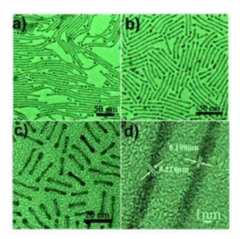
Simply changing the ratio of two chemicals in solution changes the length of ironplatinum nanowires and nanorods: transmission electron microscope images of a) 200 nm wires; b) 50 nm wires; c) 20 nm rods; d) two individual 50 nm wires. Credit: Chao Wang & Jaemin Kim/Brown University
