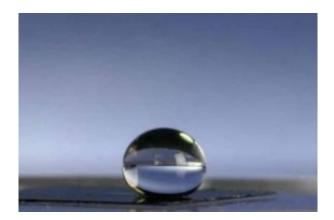
A drop of water balances perfectly on a plastic surface invented by researchers at Ohio State University. The surface is covered with microscopic fibers, and can be made to attract or repel water. The surface shown here is water repellant, so the drop can't spread out along the surface; instead, it retains its spherical shape. Credit: Photo by Jo McCulty, courtesy of Ohio State University
