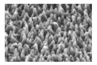
A scanning electron microscope image of plastic fibers grown on a sheet of transparent film. Ohio State University researchers have invented a technique for carpeting a surface with tiny plastic fibers. The fibers can be made to attract or repel water and oil. Credit: Image courtesy of Ohio State University
