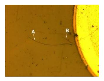
[Top] Micrograph of a complete nanowire LED with the end contact. The long nanowire (A) is about 110 micrometers long, a shorter nanowire (B) crosses it. The bright circular section is the metal post from which the nanowires are aligned. Credit: NIST
