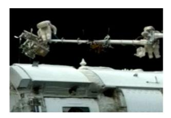
During the May 30 spacewalk, Flight Engineer Oleg Kotov (left) rides on the end of the Strela crane with a bundle of debris panels as Commander Fyodor Yurchikhin operates the controls. Image credit: NASA TV
