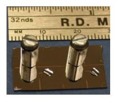
Atomic spectroscopy on a chip was achieved using this device, which features interconnected waveguides, rubidium vapor cells, and fiber-optical access. Photo courtesy of H. Schmidt
