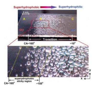
Wetability gradient: Water sprayed on a glass slide coated with a nanostructured gradient wettability film using the new NIST technique illustrates the transition from (A) superhydrophobicity to (C) superhydrophilicity. The lower image shows the magnified image of the (A) hydrophobic to (B) transition wetting region. The pink dotted line indicates the border of the superhydrophobic region, and the yellow dotted region shows a hydrophobic 'sticky' region. Credit: NIST
