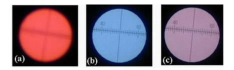
Photographs of the multi-color light emitter, 200 micrometer in diameter, taken under a microscope: the electrical current was 0.02 mA (a), 1 mA (b) and 2.5 mA (c), respectively. The violet color in (c) is a result of mixing the red and the blue.
