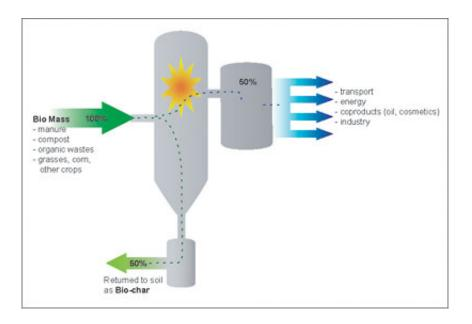
When bioenergy is produced by pyrolysis (low-temperature burning without oxygen), it produces biochar, which has twice as much carbon in its residue than that from other sources. This makes bioenergy carbon-negative and improves soil health. Credit: Cornell University
