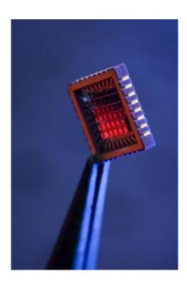
The world's first silicon spin-transport devices, fabricated and measured in Ian Appelbaum's lab at the University of Delaware. More than 25 individual silicon spin-transport devices are represented, one within each tiny wire grid, on this ceramic chip holder. Credit: Jon Cox, University of Delaware
