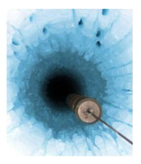
The IceCube telescope's optical detectors are deployed in mile-and-a-half deep holes in the Antarctic ice. Credit: James Roth, University of Delaware
