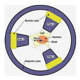
Scheme of the micromechanical experiments. Magnetic poles (6  $\mu$ m wide, 20  $\mu$ m separation) generate a force on a paramagnetic bead positioned in the nucleus of a HeLa cell. Electric coils allow the control of amplitude and direction of the force. Magnetic yoke and electric coils are not to scale. Credit: University of Twente
