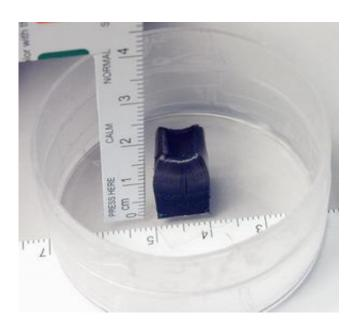
University of Cincinnati researchers have created the longest carbon nanotubes in the world. Grown in arrays that are centimeters long, the fibers catch the light as thin striations. Credit: V. Shanov, M. Schulz, University of Cincinnati
