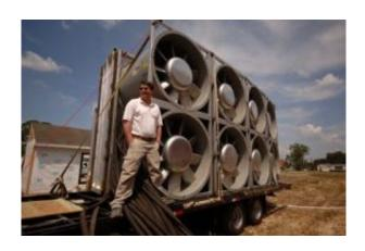
University of Florida wind engineering researcher Forrest Masters stands on a newly completed, fully portable hurricane wind simulator on May 29, 2007.
