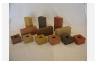
Researchers have developed bricks that look and perform like normal bricks yet are crafted from fly ash, a waste produced by coal-fired power plants. Credit: Henry Liu, FPC
