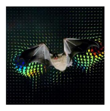
On the cover of Science: A bat, Glossophaga soricina, in flight in a wind tunnel at Lund University, Sweden. The velocity field induced by the wingbeat is shown superimposed and to scale. The bat wake reconstructions have features that have not been observed in similar-sized birds. Membranous and feathered wings of natural and engineered flyers may have significantly different aerodynamic properties. Credit: Lund University, Sweden
