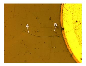
Micrograph of a complete nanowire LED with the end contact. The long nanowire (A) is about 110 micrometers long, a shorter nanowire (B) crosses it. The bright circular section is the metal post from which the nanowires are aligned.
