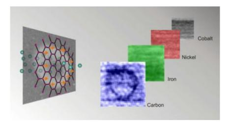
A carbon film is hit by a high-energy proton beam, causing the magnetic moments of the atoms to align around the beam impact area and creating a ring-shaped magnetic pattern that can be imaged with a magnetic-force microscope. The X-ray microscope can also be tuned to "scan" the sample for magnetism associated with other elements. The absence of a ring pattern in scans for cobalt, nickel and iron prove that the sample contains only carbon. Credit: SLAC
