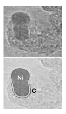
Environmental transmission electron microscopy image sequence of carbon nanofibre growth. Drawings (lower row) indicate schematically the Ni catalyst deformation and C-Ni interface. Credit: University of Cambridge
