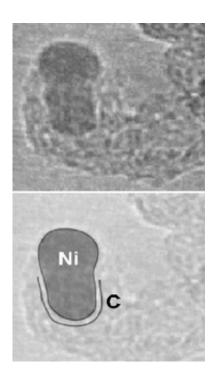
Environmental transmission electron microscopy image sequence of carbon nanofibre growth. Drawings (lower row) indicate schematically the Ni catalyst deformation and C-Ni interface. Credit: University of Cambridge
