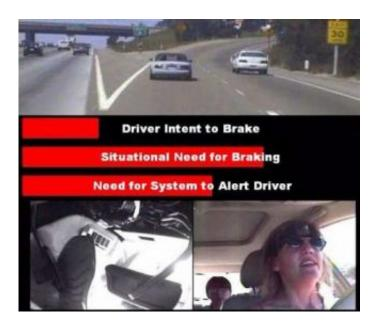
Over the past several years, scientists working in the area of intelligent vehicles have developed predictive braking systems to help prevent rearend collisions. When your car gets dangerously close to the car in front of you, the system can warn you or automatically put on the brakes.
