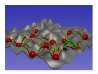
Illustration of a Coulomb glass system: Electrons (red) in a random landscape, interacting with each other (yellow-orange lines). Noise of the resistance of the system is created by collective "hopping" of the electrons (green arrow). Credit: Argonne National Laboratory
