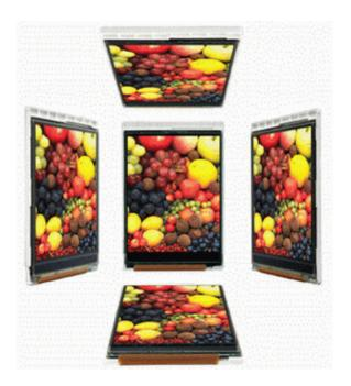
Sharp has succeeded in developing a new LCD for mobile equipment such as mobile phones. The new LCD features the industry's highest contrast ratio of 2,000:1, a wide viewing angle of 176 degrees that is top class in the industry, and a high-speed response time of 8 ms.
